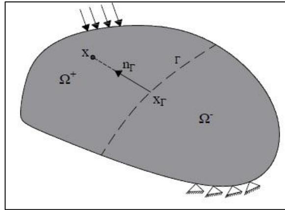
Figure 1. Body domain crossed by crack discontinuity.
