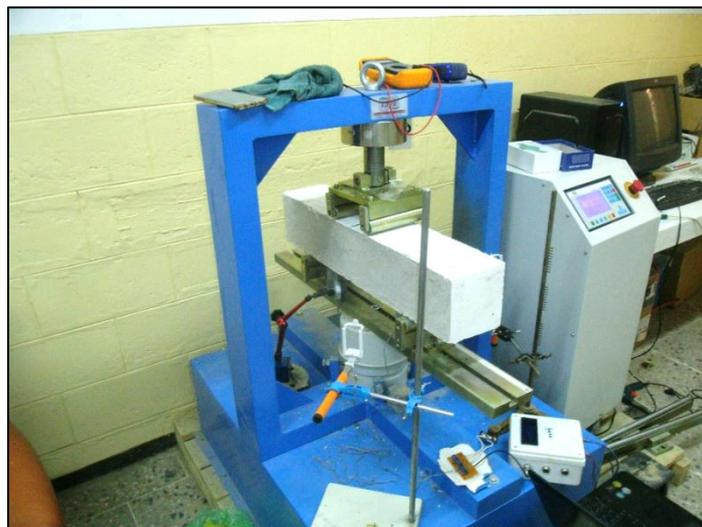
**Plate 1.** Laboratory testing machine for the plain concrete beam.
