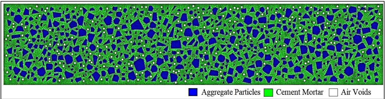
**Figure 3.**Meso-scale numerical model for the plain concrete beam.
