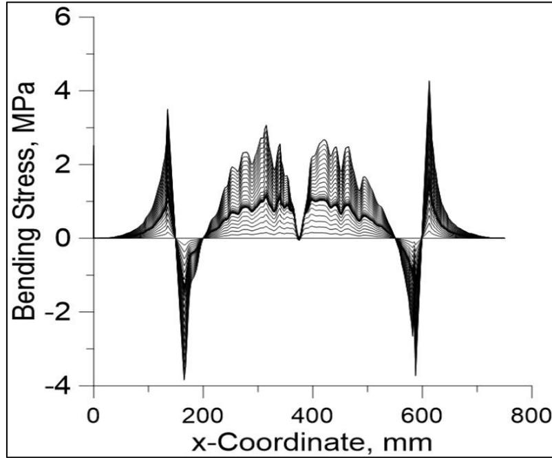
Figure 5. Meso-scale bending stress diagram along the concrete beam.
