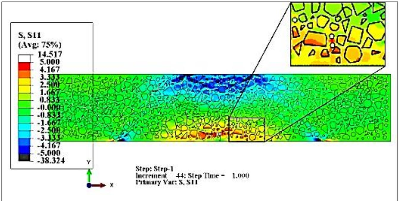
Figure 6. Meso-scale bending stress diagram along the concrete beam.
