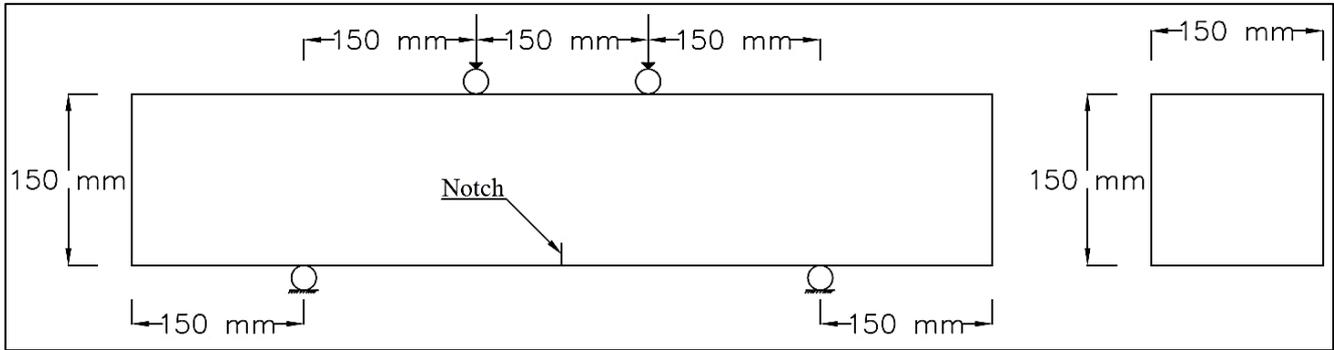
Figure 2. Loading system of the concrete beam model.
