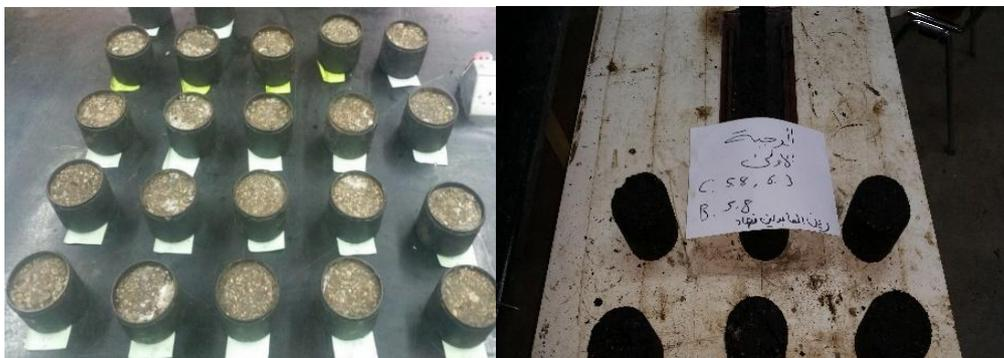
**Figure 2.** Part of the prepared cylindrical specimen for indirect tensile strength ratio test and index of retained strength.
