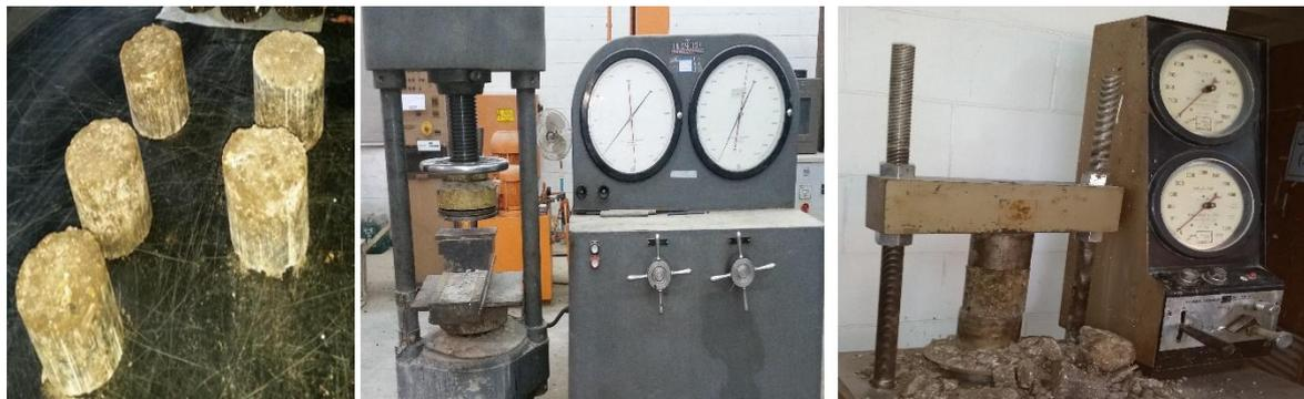
**Figure 4.** Part of the prepared specimens and the test apparatus (index of retained strength).
