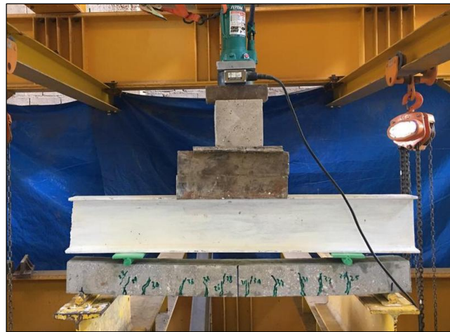
Figure 8. Cracks Propagation in control beam specimen.
