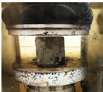
(a) Testing concrete cubes
