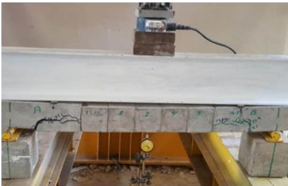
Figure 10. Cracks propagation and failure mode of beams with no adhesion at segments interface.
