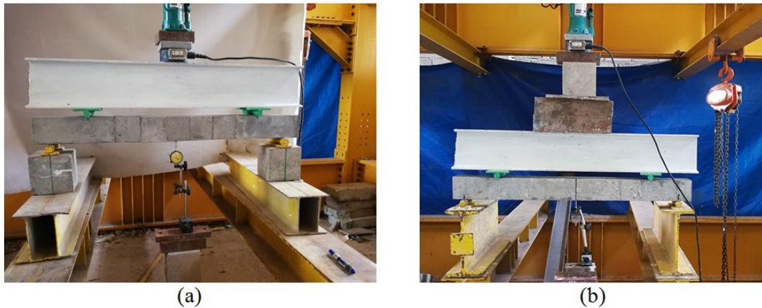
Figure 6. Specimens testing, (a) segmental beams (b) reference beam.
