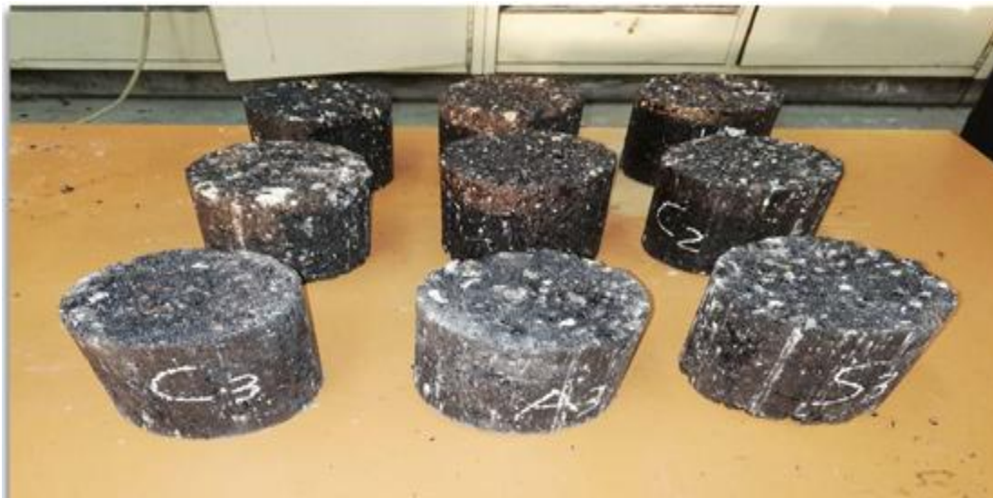
Plate 2 . Set of prepared compressive specimens.
