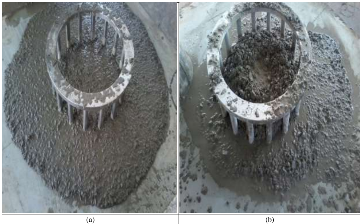
Figure 1. J ring test (a) for Ref. mix 2 and (b) for Mix8.
