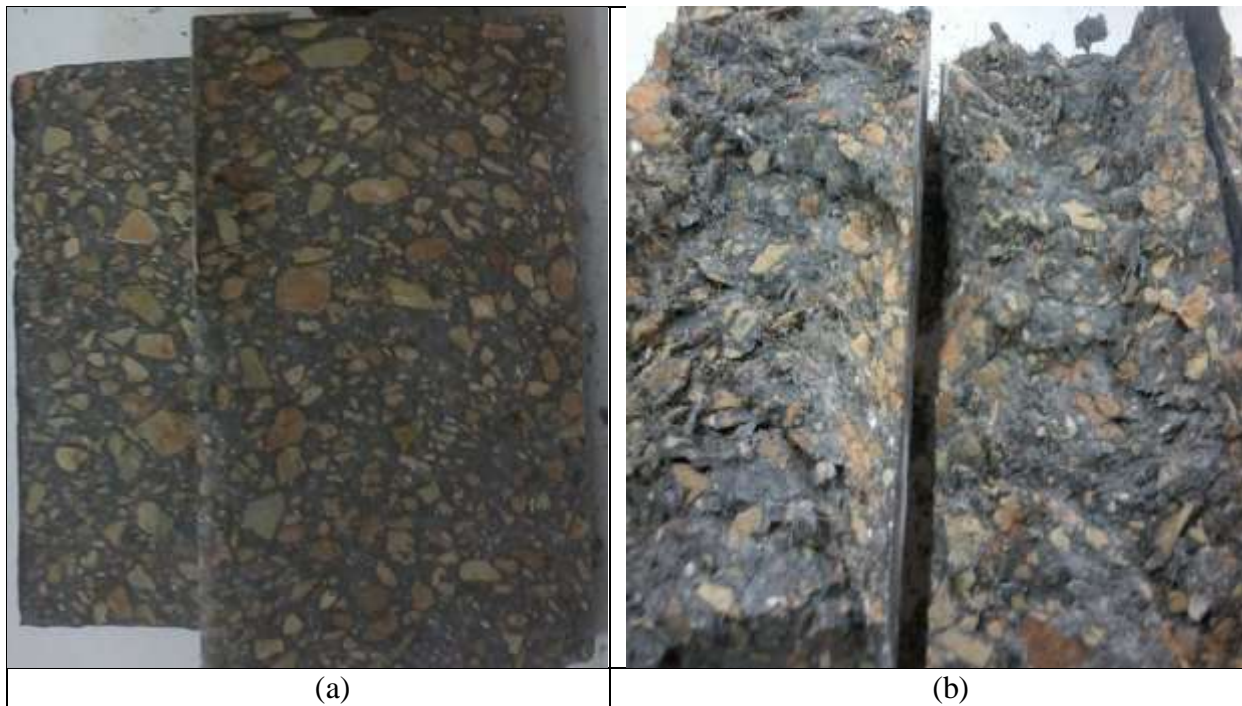
Figure 5. Failure plane of splitting tensile test specimen (a) for Ref. mix 1 and (b) for Mix 4.
