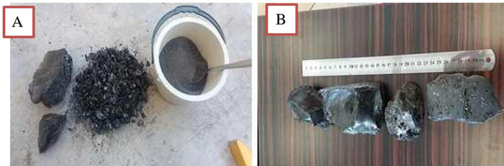
**Figure 1.** The used steel slag in the laboratory tests, A- Large particle size, B- Crushed and powdered.
