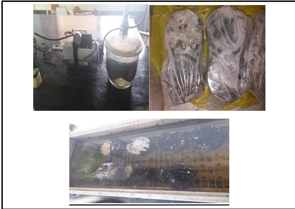
Figure 2. Part of the core conditioning process.
