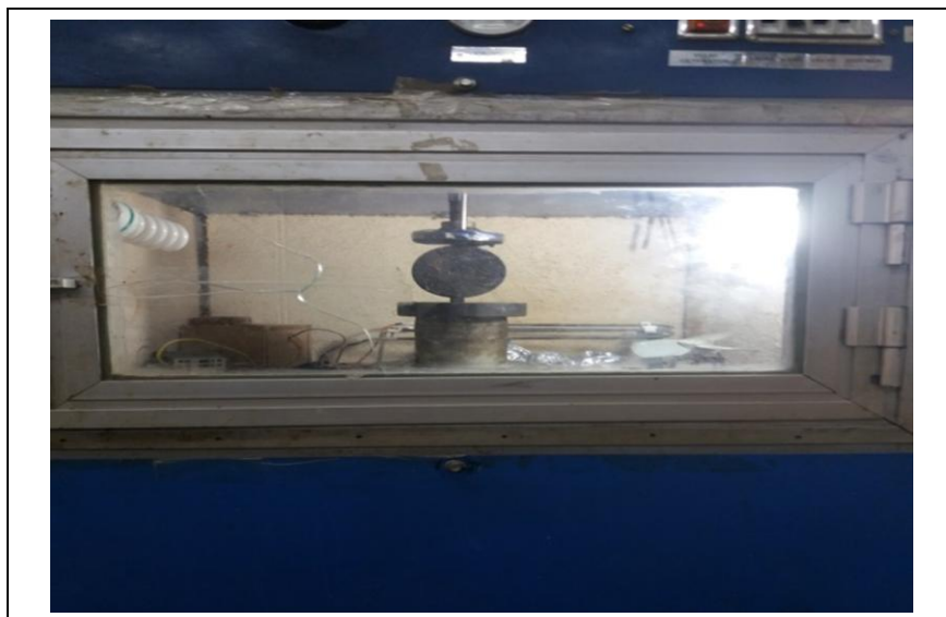
Figure 3. Pneumatic repeated load system.
