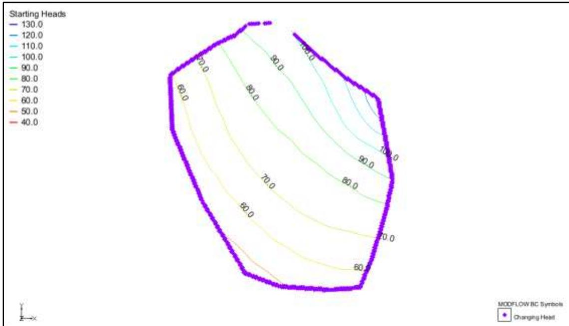
Figure7. Boundary condition and starting head of Turssaq alluvial fan.
