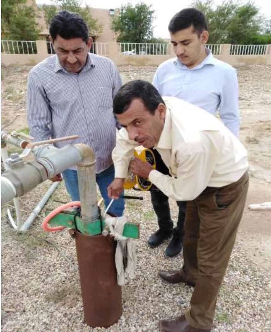
**Figure10.** Measure the groundwater table in the well.
