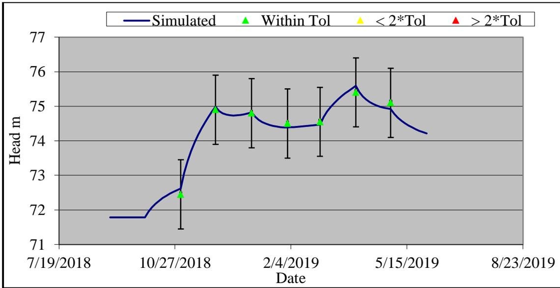
Figure 11. Measured and simulated heads in Turssaq Alluvial, Fan W18.
