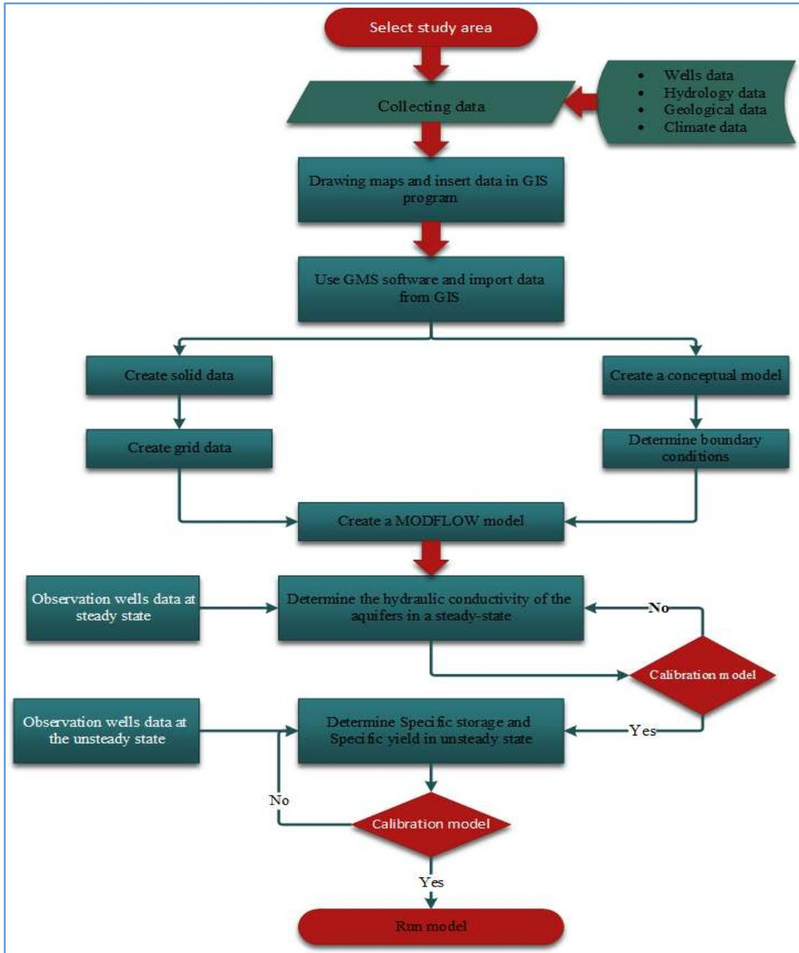
**Figure2.** The methodology of developing the conceptual model groundwater simulation.
