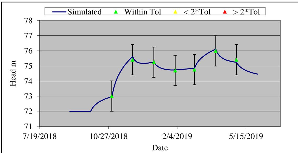
Figure 12. Measured and simulated heads in Turssaq Alluvial Fan, W24.
