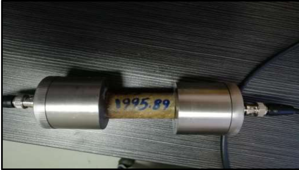
Figure 2. James instrument ultrasonic device used for measuring the sonic waves velocities.
