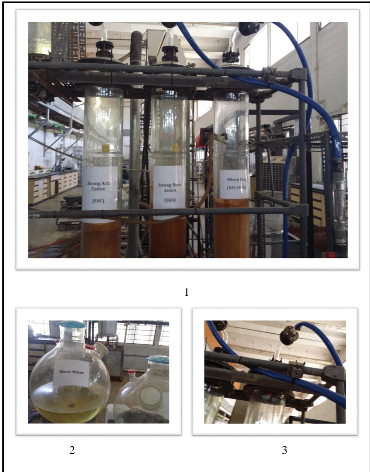
Figure 8,a. Photograph of Ion exchange continuous equipment.
