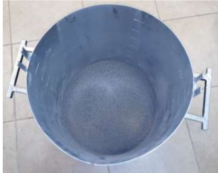
Figure 3. The soil container used for pile modeling.
