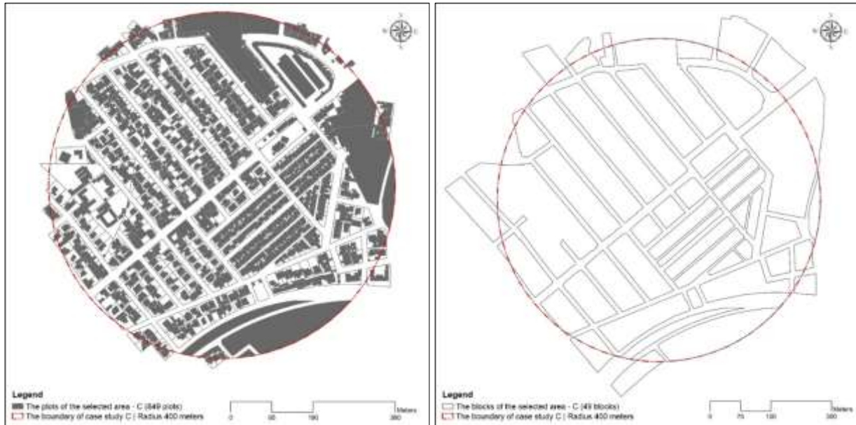
Figure 2. (Left) The paralleled pattern. Both the spatial configuration of plots and blocks are regular. (Right) The paralleled pattern illustrates blocks arrayed in a parallel way opposite each other on the longest side. Source: Drawn by the author based on the georeferencing aerial imagery and Base Map Baghdad authorised by (R.S.GIS.U, 2017).
