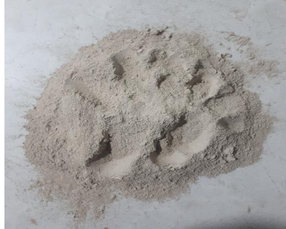
Figure 3. Mechanism of crushing the concrete Figure 4. Concrete demolishing waste (CDW). demolishing waste (CDW).
