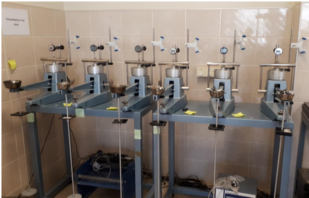
Figure 9. Oedometer apparatuses (swelling pressure test).
