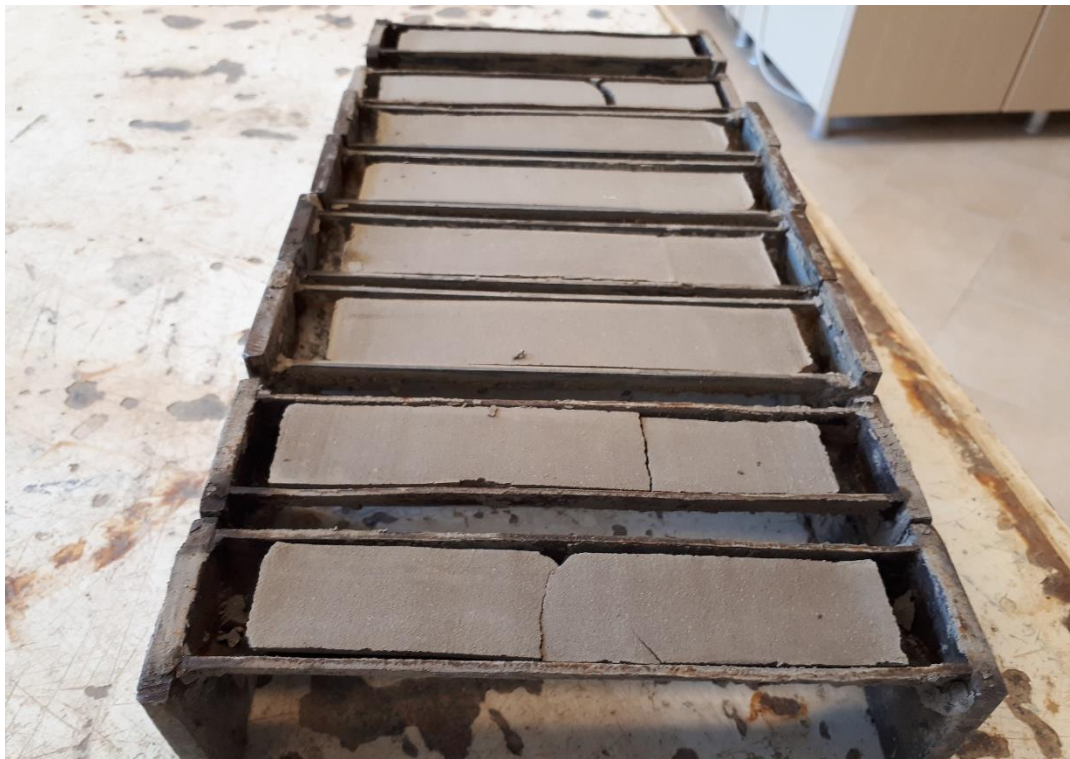
Figure 7. Linear Shrinkage test samples.
