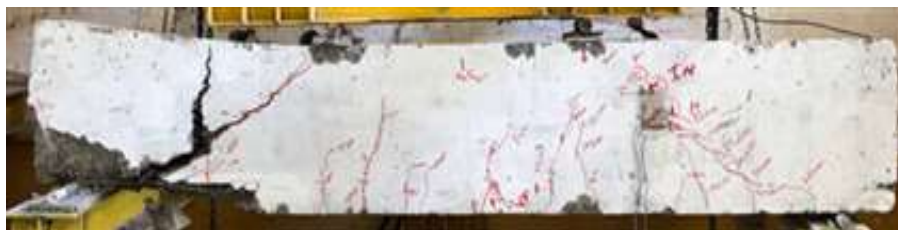
Figure 10. crack patterns of the solid beam.
