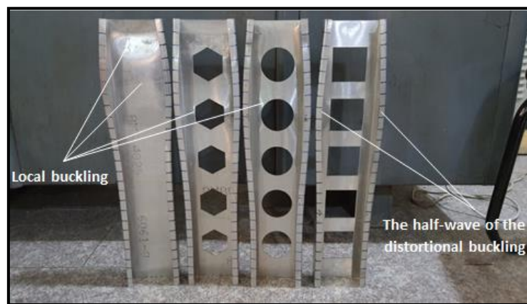
Figure 9. Specimens after buckling test under compression loading.
