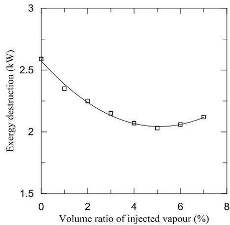
**Figure 7.** The variation of total exergy destruction vs volume ratio of injected vapour.
