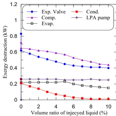
**Figure 9.** The variation of components exergy destruction vs volume ratio of injected liquid.
