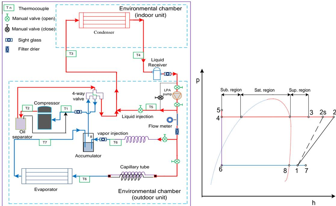
**Figure 1.** Schematic and P-h diagrams of heat pump cycle with LPA and hybrid injection technologies.
