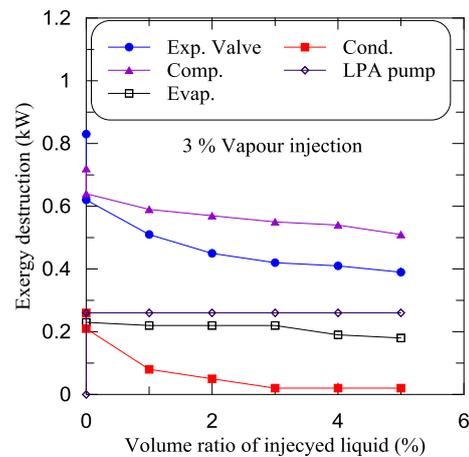
**Figure 14.** The variation of components exergy destruction vs volume ratio of hybrid injection at (3% vapour injection).
