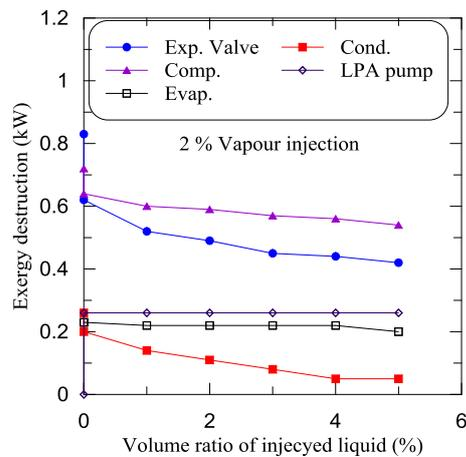
**Figure 13.** The variation of components exergy destruction vs volume ratio of injected liquid at (2% vapour injection).
