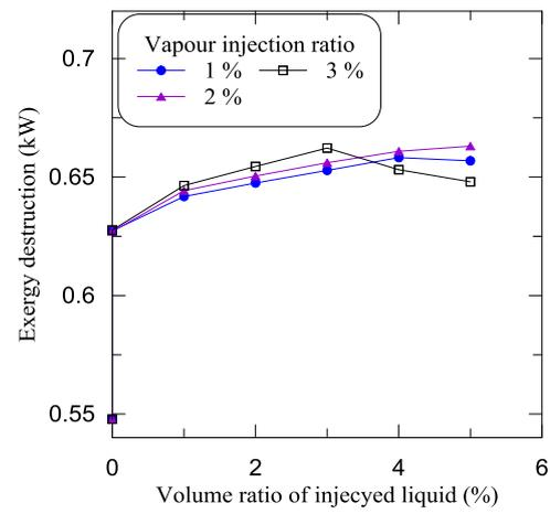
**Figure 15.** The variation of total exergy efficiency vs volume ratio of hybrid injection.
