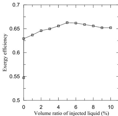
**Figure 11.** The variation of total exergy efficiency of heat pump system vs volume ratio of injected liquid.
