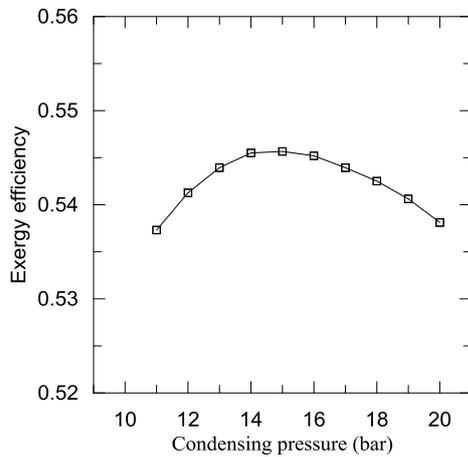
**Figure 5.** The variation of total exergy efficiency vs condensing pressure.
