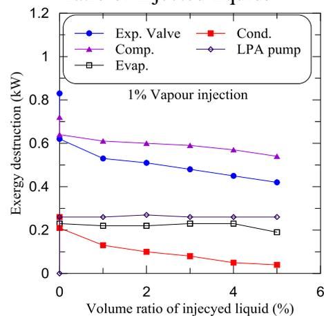
**Figure 12.** The variation of components exergy destruction vs volume ratio of injected liquid at (1% vapour injection).
