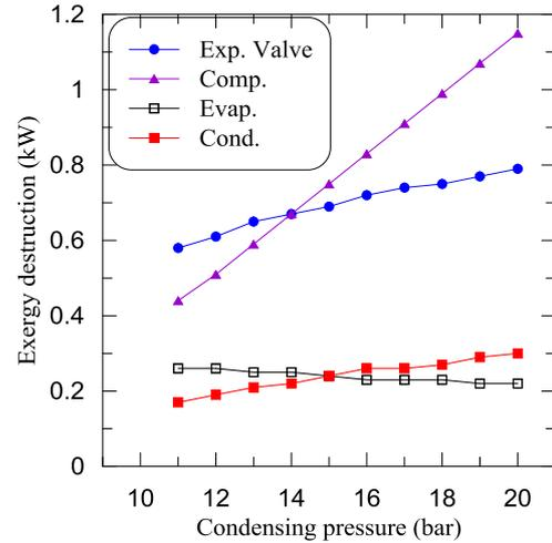
**Figure 4.** The variation of exergy destruction of components vs condensing pressure.
