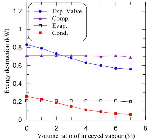
**Figure 6.** The variation of components exergy destruction vs volume ratio of injected vapour.
