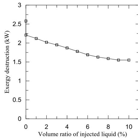
**Figure 10.** The variation of total exergy destruction of heat pump system vs volume ratio of injected liquid.
