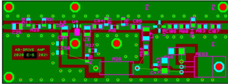
Figure 5. The layout of the RF Amplifier.
