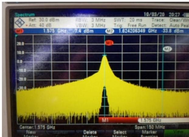
**Figure 12.** Amplifier output signal.
