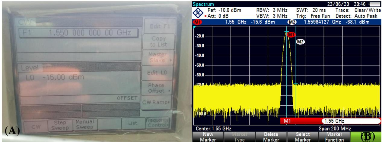
**Figure 9.** (A) signal generator, (B) the signal spectrum that appears on the spectrum analyzer.
