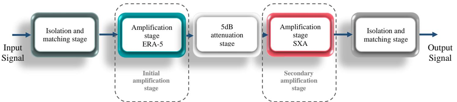
Figure 4. Block diagram of the RF Amplifier according to the first model.
