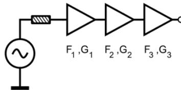
**Figure 1.** A diagram of a multistage receiver system.
