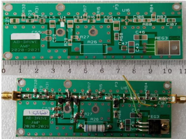
Figure 6. Printed circuit board manufactured according to the first model.
