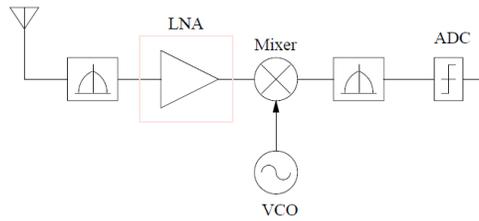
Figure 2. Typical architecture of a radio receiver (LIU, 2011).
