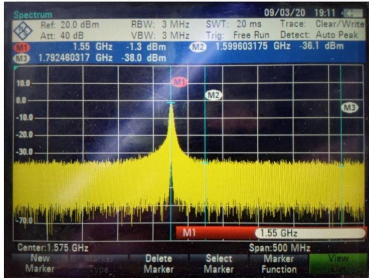
**Figure 10.** Power amplifier output signal.
