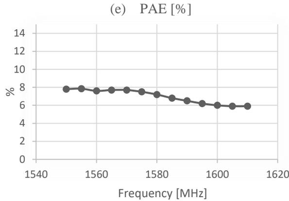
**Figure 11.** (a) - signal-to-noise ratio, (b) - output signal capacity, (c) - noise figure, (d) - amplifier gain, (e) - Power Added Efficiency vs frequency.
