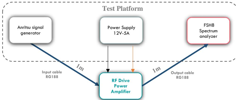
Figure 3. Block diagram of the test platform.
