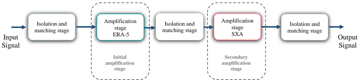
Figure 7. Block diagram of the RF Amplifier according to the second model.
