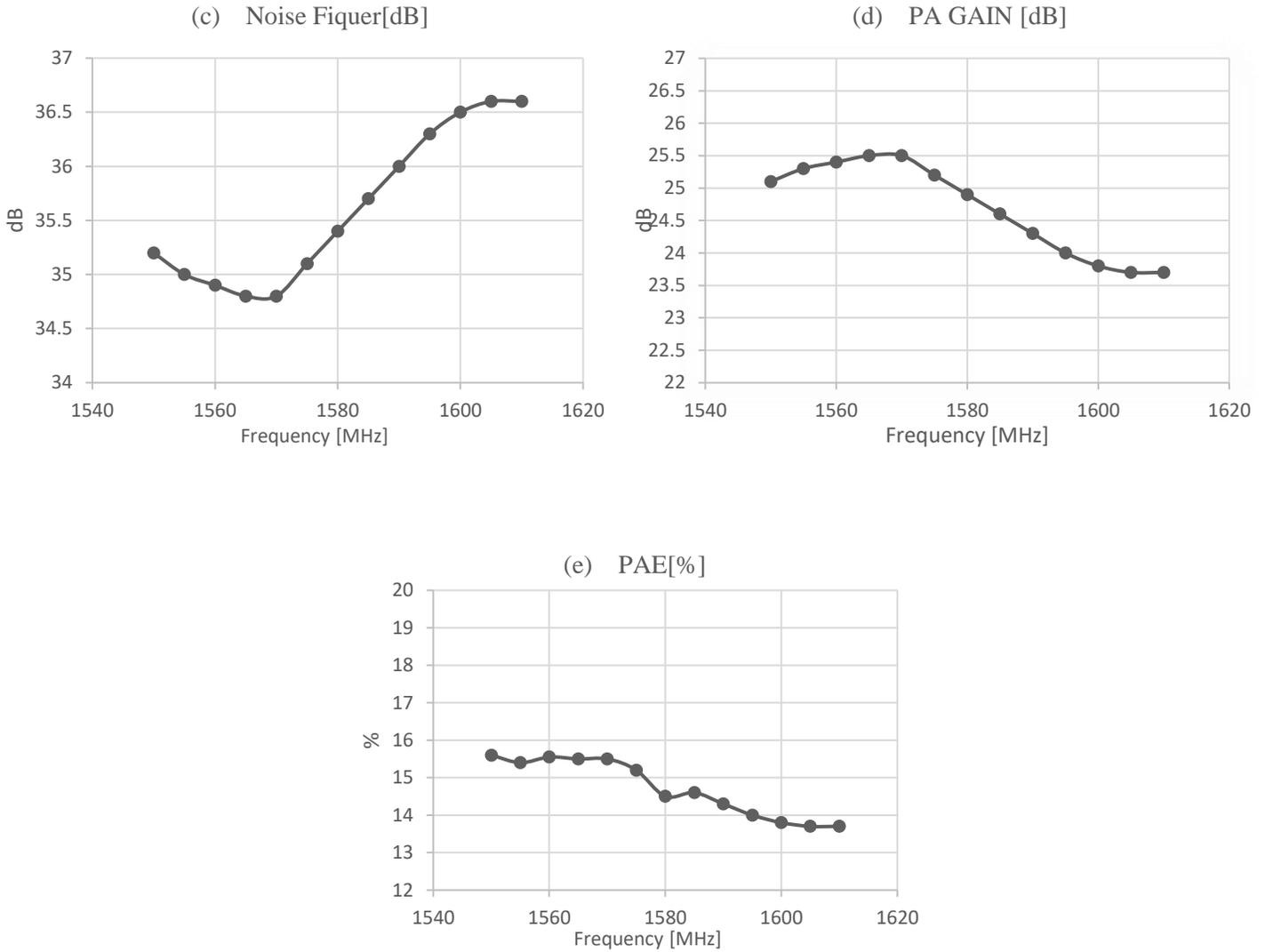
Figure 13. (a) - signal-to-noise ratio, (b) - output signal capacity, (c) - noise figure, (d) - amplifier gain, (e) - Power Added Efficiency vs frequency
