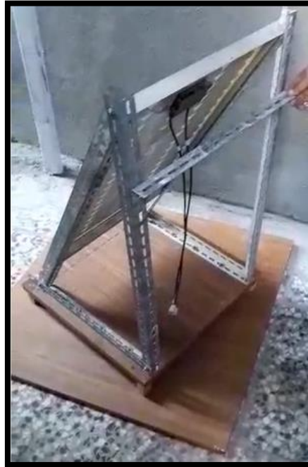
Figure 3. Manual orientation mechanism and holder structure.
