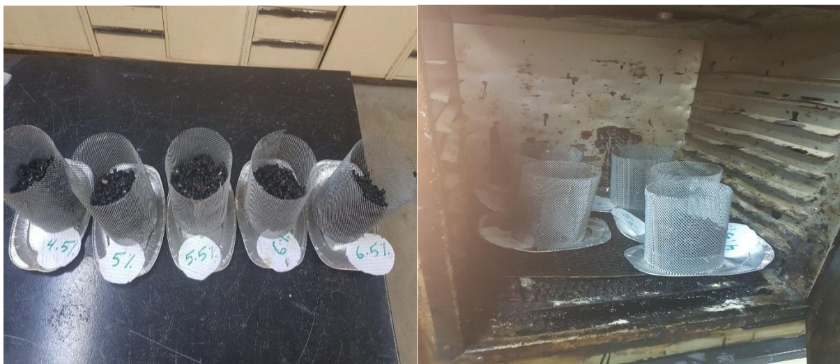
Figure 4. Drain down test.
