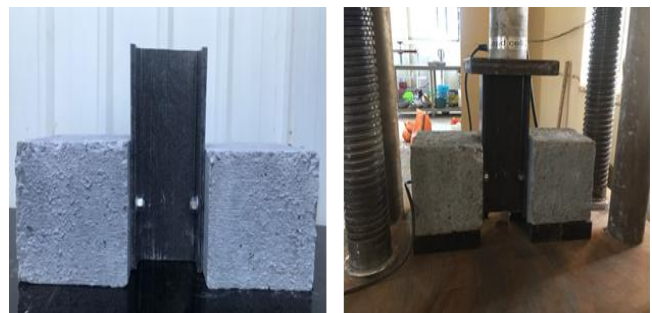
Figure 6. Shear connection test setup.
