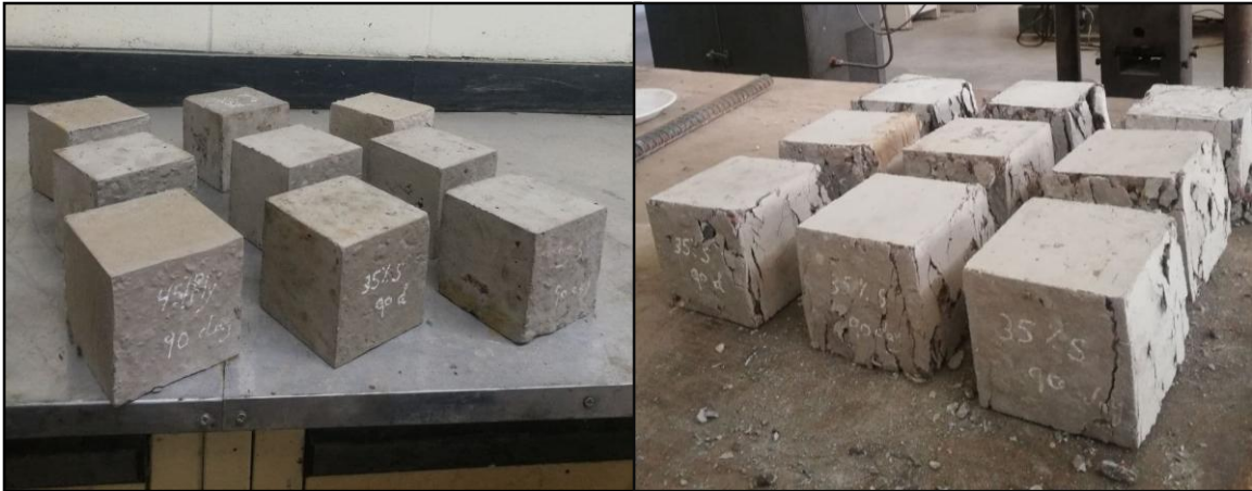
Figure 2. Geopolymer cubes before the compressive test (left), after the compressive test (right).
