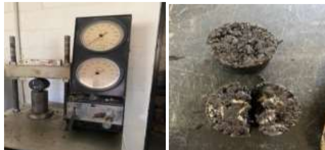
Figure 3. Indirect Tensile Strength test for WMA specimen
