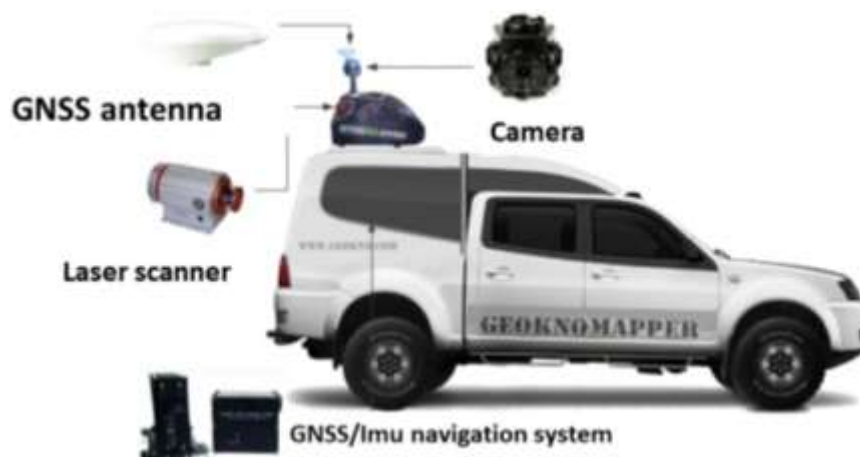
Figure 7. The components of the MLS system (Lohani and Yadav, 2018) .
