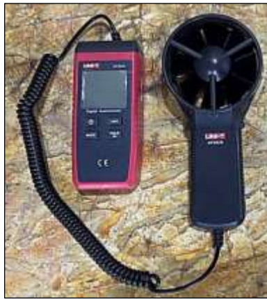
Figure 6. Vane type of digital anemometer UT363S.
