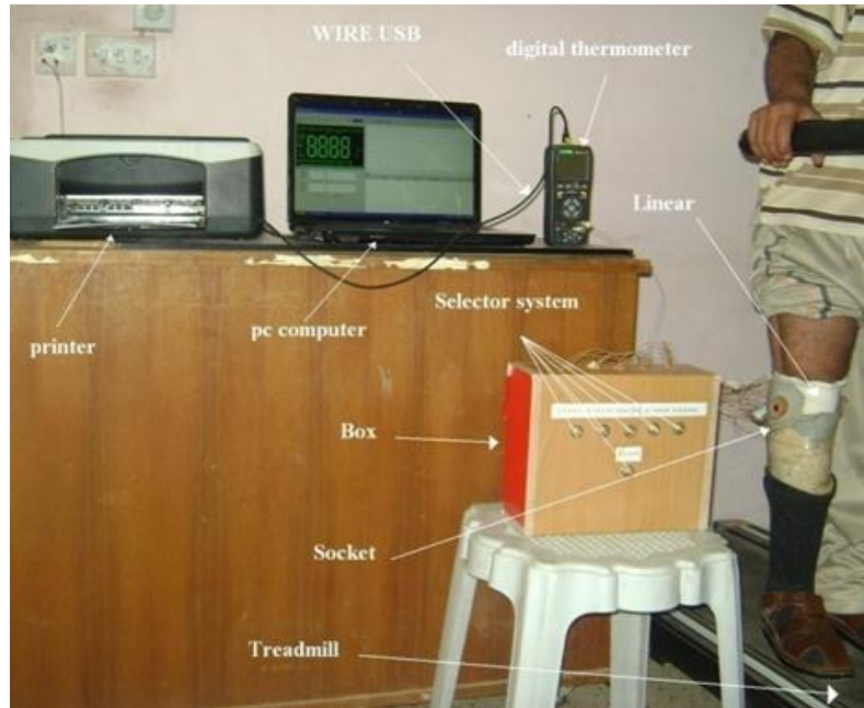
Figure 6. Trans-tibial amputee during IP test.
