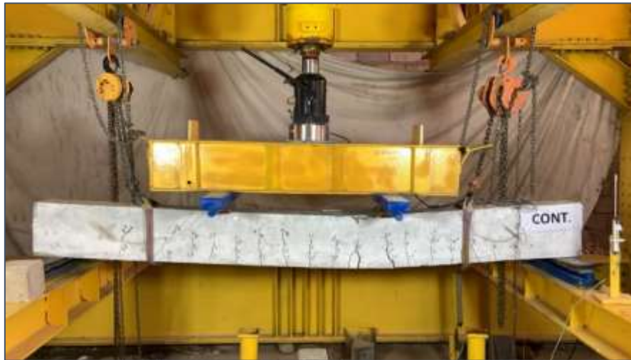
Figure 9. The Failure pattern of Cont. beam.
