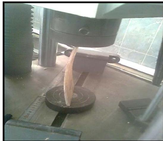
Fig. (4 b): Buckling test of F-S-F-S laminates
