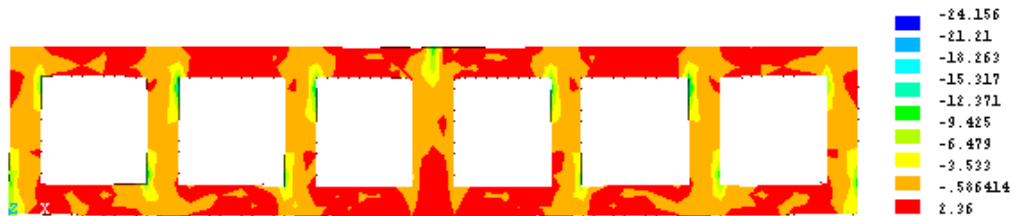
Fig. 21 Stress distribution in Y-direction for VER1, (N/mm 2 ).
