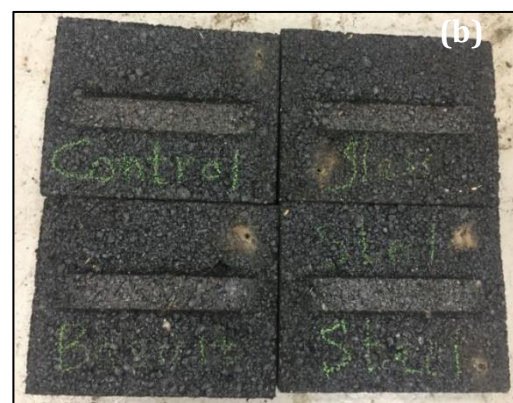
Figure 4. (a) Wheel Tracking Device, (b) Slabs After Wheel Track Test
