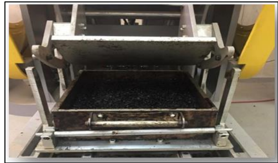
(b) Slab during the compaction
