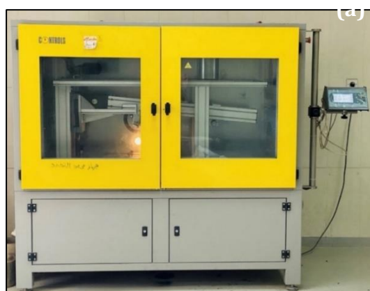
Figure 4. (a) Wheel Tracking Device, (b) Slabs After Wheel Track Test
