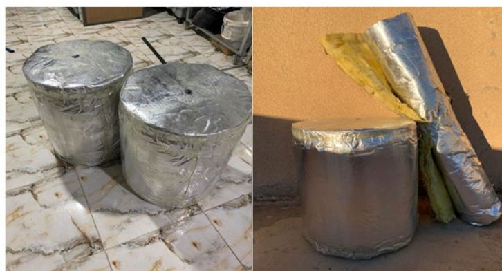
Figure 4. Insulated Storage tank.
