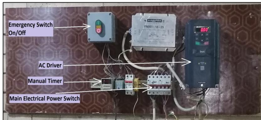
Figure 6. The electrical board details of the model.
