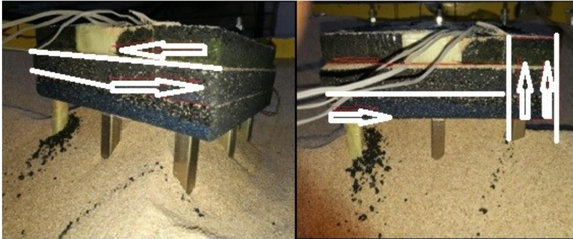
**Figure 17.** The deformation behavior of the rubber pads layers (thickness is 6cm) after the shaking loading effect.
