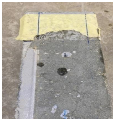
Figure 10. The failure mode of the L100W25 specimen
