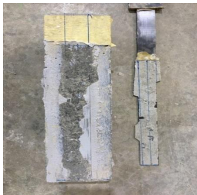
Figure 7. The failure mode of the L200W25 specimen
