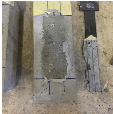
Figure 6. The failure mode of the L150W25 specimen
