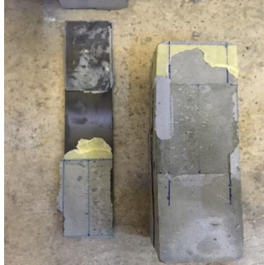
Figure 9. Failure mode of L100W50 specimen
