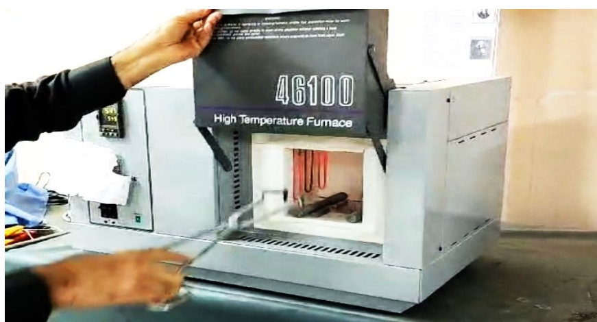
Figure 4. High-Temperature Furnace “Thermolyne model box Furnace” used for this study's heat treatment purpose.
