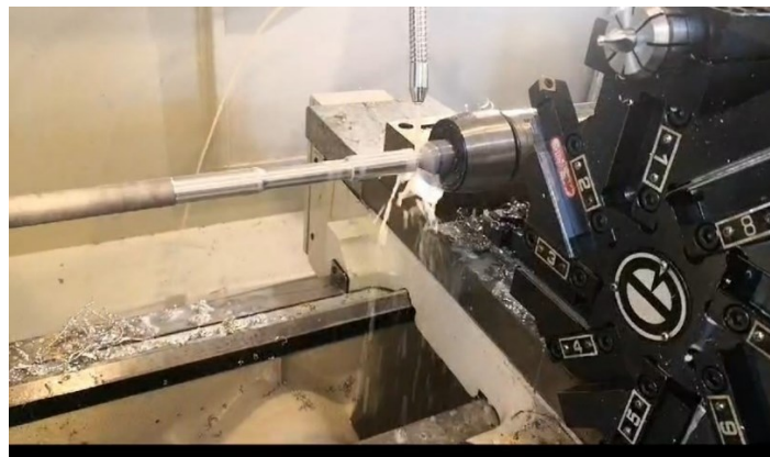
Figure 2. Experimental work on the Al alloy 2024 to make tensile test specimens machined by CNC lathe machine operation.
