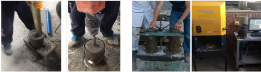
Figure 4. Different RCC laboratory compaction methods (Şengün et al., 2019)
