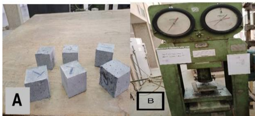
Figure 2. Compressive strength test: (A) sample for test; (B) compressive strength device.
