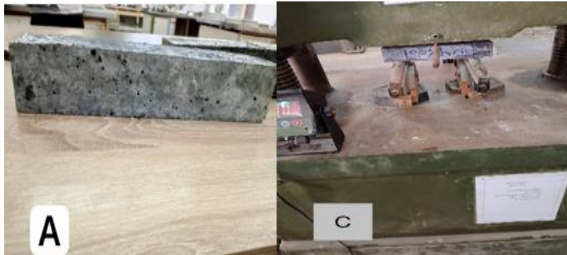
Figure 3. Flexural strength test: (A) sample for test; (C) sample under test.
