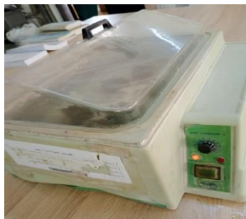
Figure 1. Water bath device for curing the samples of MRPC.
