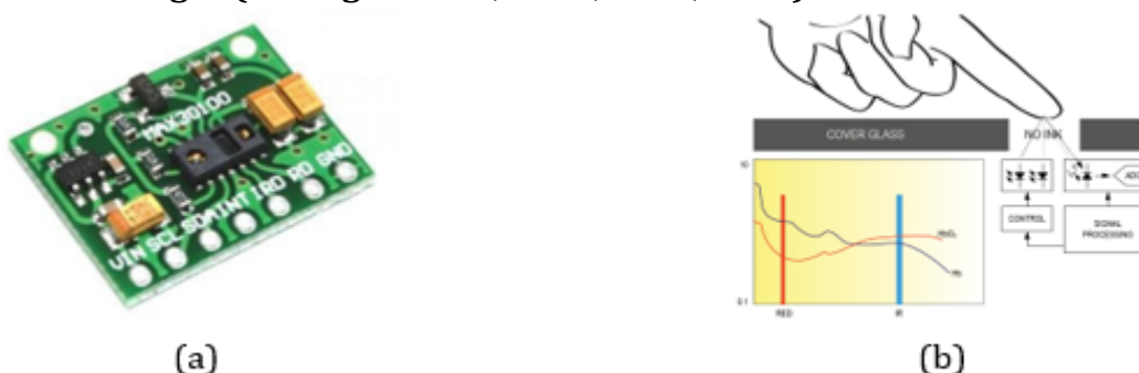
Figure 3. MAX30100 Sensor (a) The board of the sensor (b) The block diagram of the sensor.
