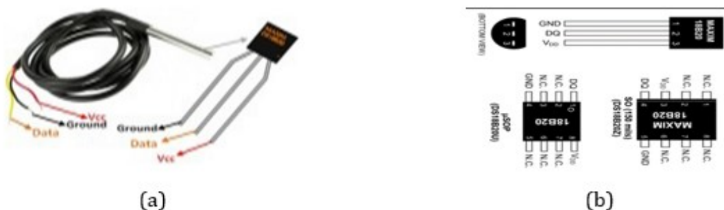
Figure 4. The used body temperature (a) The DS18B20 Sensor (b) The pin configuration ( Mohammed et al., 2014 )
