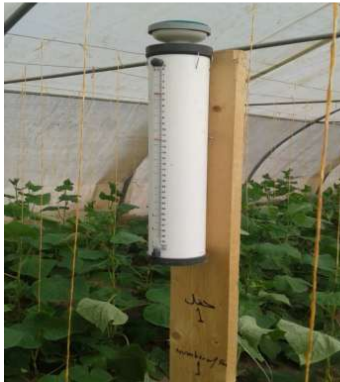
Figure 2. Location of the atmometer apparatus in the cucumber's greenhouse.
