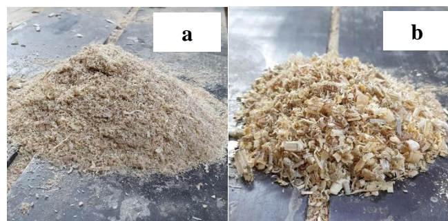
Figure 1. Sawdust wastes with different particle sizes (a) fine (b) coarse
