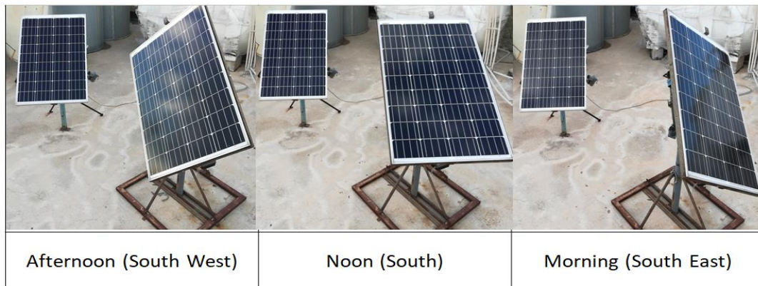
Figure 4. Fixed and Tracking PV Test Systems.
