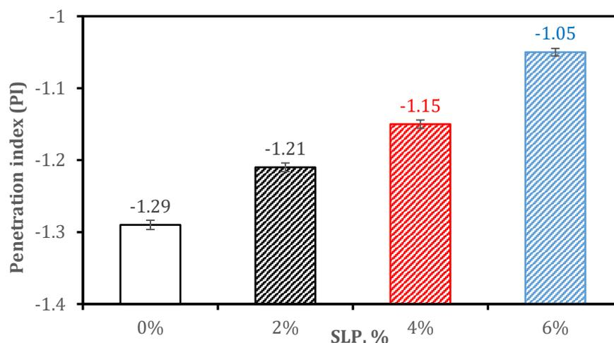
**Figure 11.** Effect of soda lignin content on the penetration index.
