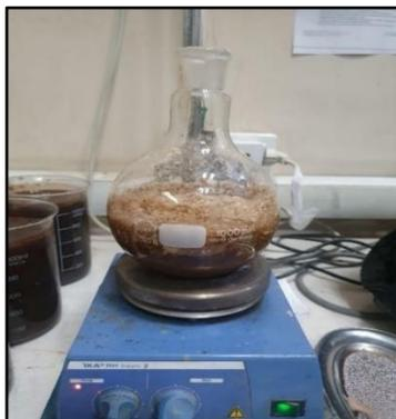
(b) Mixing wood with alkaline solution
