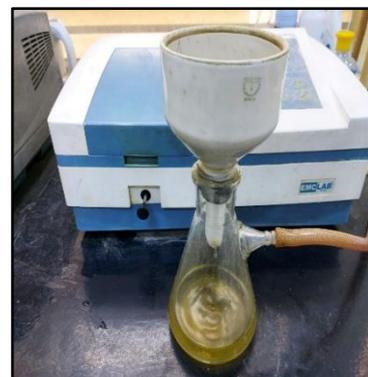
(c) Filtering the solution by vacuum filtration apparatus
