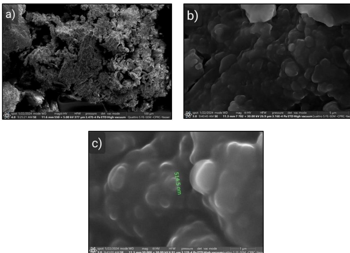
**Figure 5.** SEM micrographs of soda lignin, (a) with a magnification of 500 $\times$ , (b) with a magnification of 7000 $\times$ , (c) with a magnification of 30000 $\times$ .
