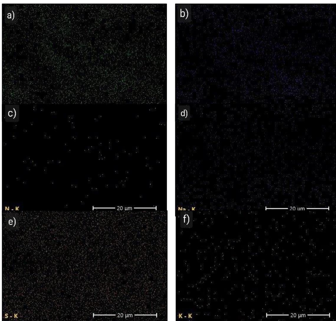
**Figure 6.** EDX elements map of soda lignin, (a) C element distribution, (b) O element distribution, (c) N element distribution, (d) Na element distribution, (e) S element distribution, (f) K element distribution, continued.
