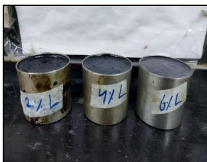
(a) Penetration test samples
