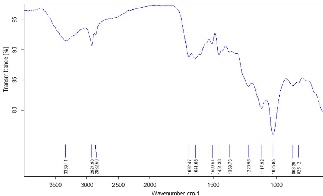
**Figure 4.** FTIR spectra of soda lignin.
