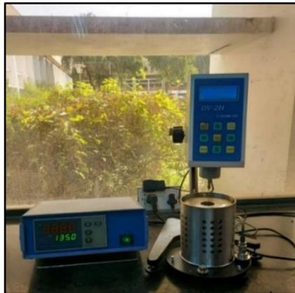
**Figure 3.** Rotational viscometer.
