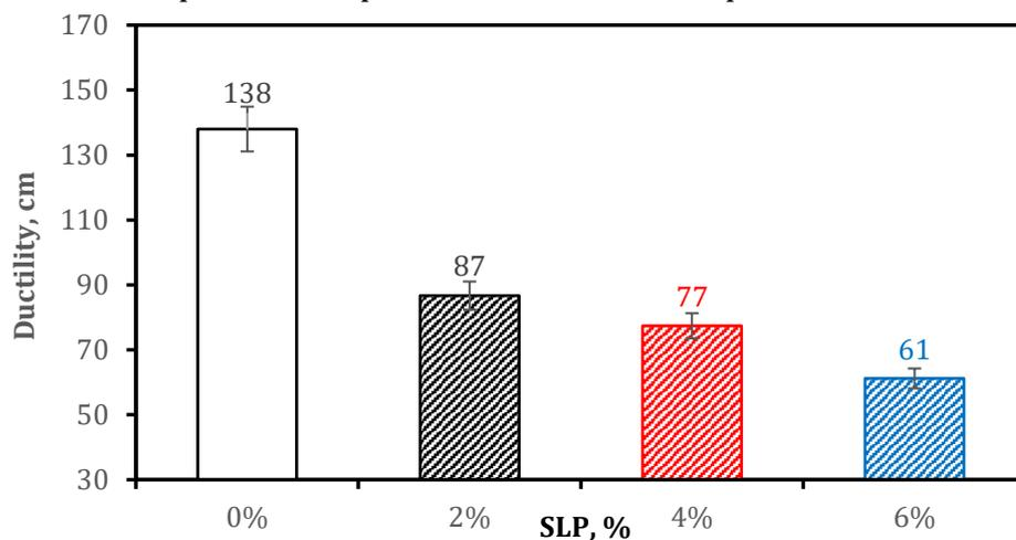
**Figure 10.** Effect of soda lignin content on the ductility.
