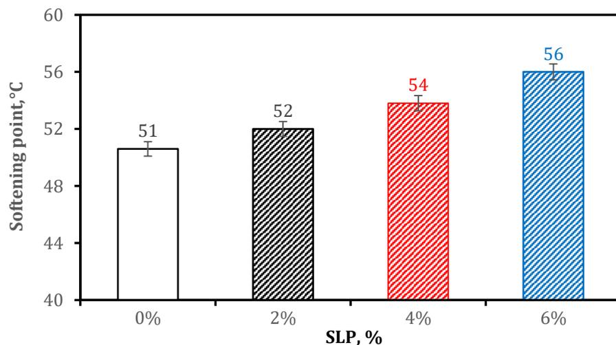
**Figure 9.** Effect of soda lignin content on the softening point.
