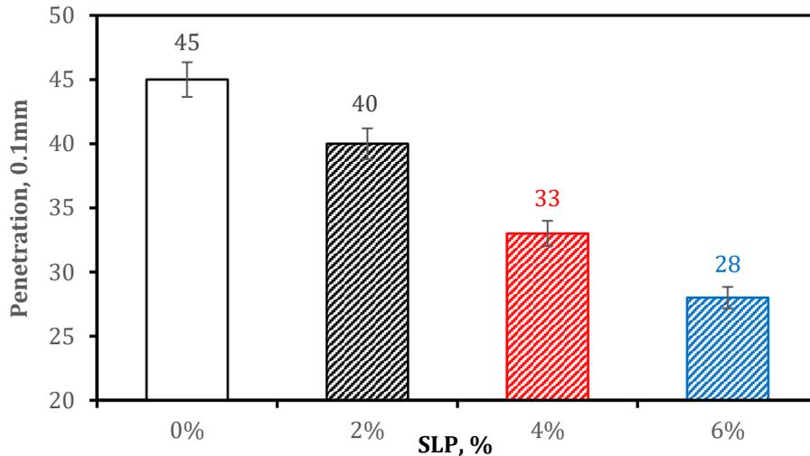
**Figure 7.** Effect of soda lignin content on the penetration at 25°C.
