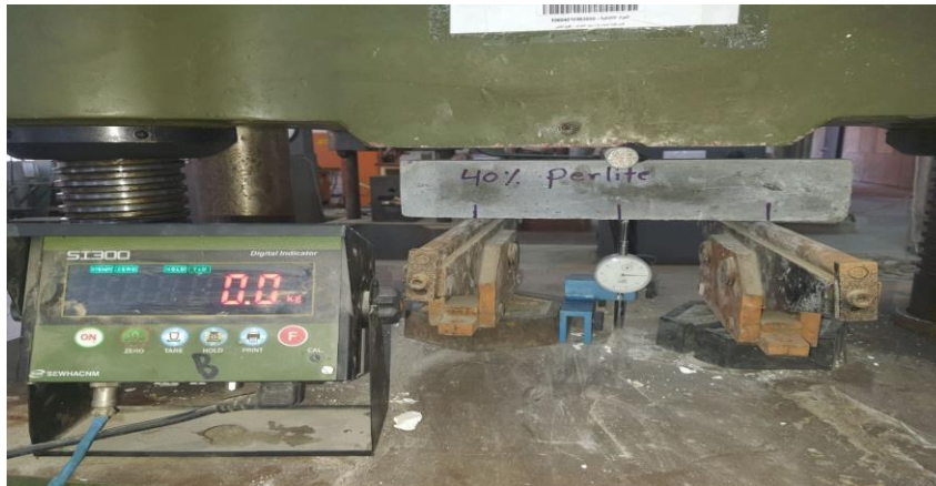
Figure 13. Flexural strength test
