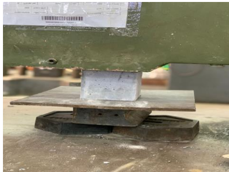
Figure 9. Compressive strength Test.
