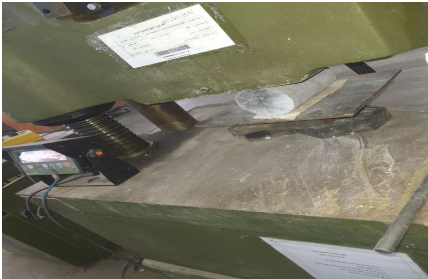
Figure 16. Splitting tensile strength test
