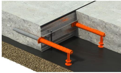
Figure 3. An example of contraction joints (Mulders, 2024)
