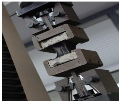
Figure 10. Setting up of bonding test ( Wagner, 2024 )
