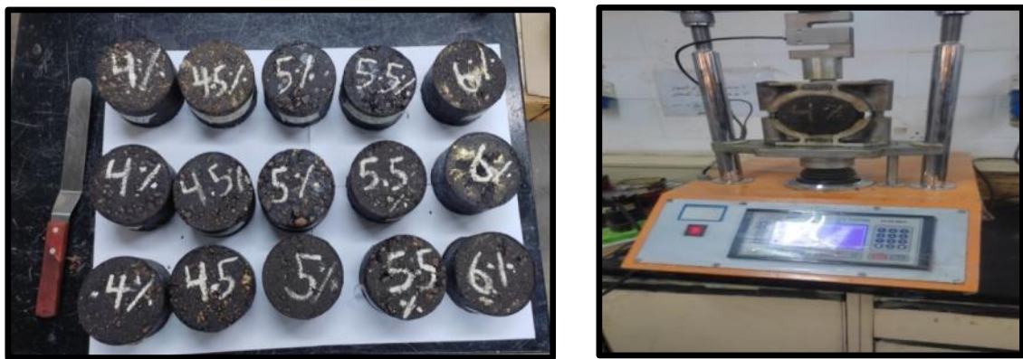
Figure 9. The specimens and Marshall test.
