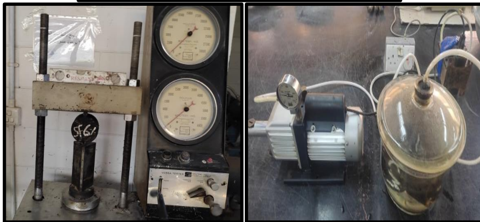
Figure 12. The indirect tensile strength test.
