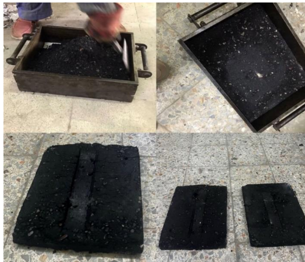
Figure 6. Samples of slabs used in wheel tracking test.
