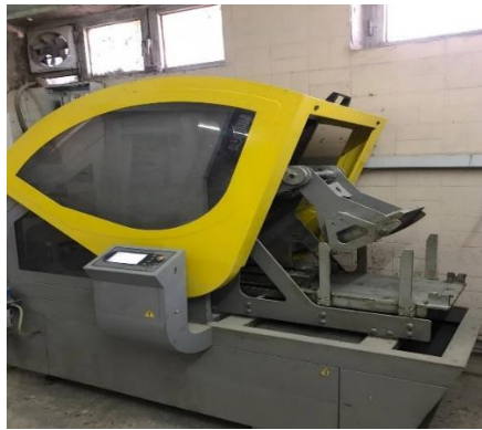
Figure 5. Roller compactor device.
