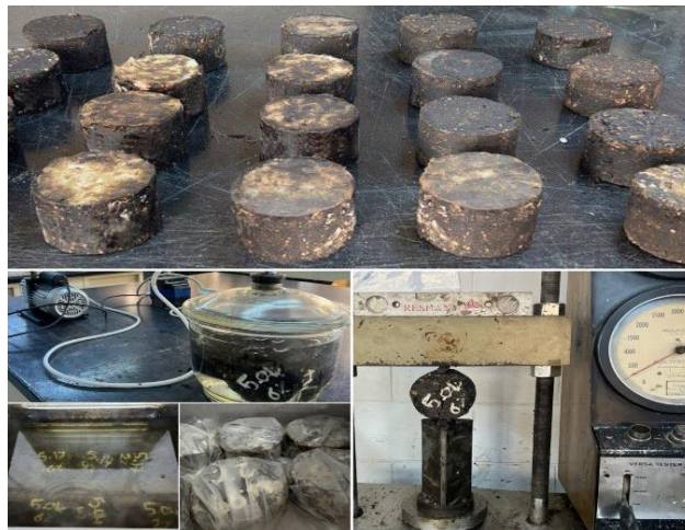
Figure 5. The testing sequences for indirect tensile strength.
