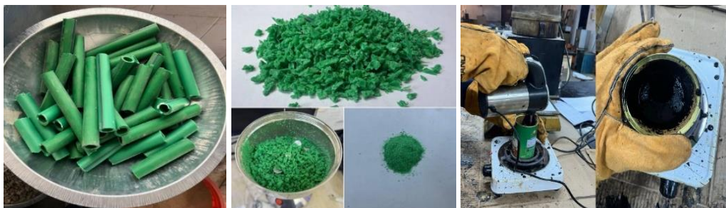
Figure 2. Polypropylene Polymer waste crushed and mixed particles.
