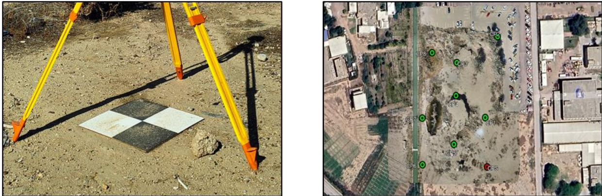
Figure 7. Ground control points, (Left) GCPs targets, (Right) distribution of the points in the site (the green points are measured in RTK mode while the red colored are measured in static mode).
