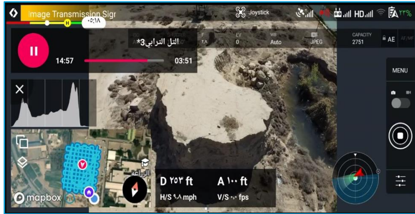
Figure 5. Flight progress and capturing of images by drone-link mobile application.
