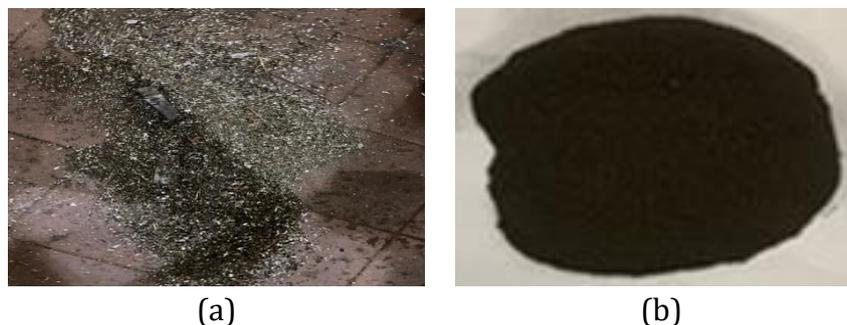
**Figure 1.** (a) Chips of mild steel, (b) Ground and sieved 100- $\mu\text{m}$  mild steel particles.
