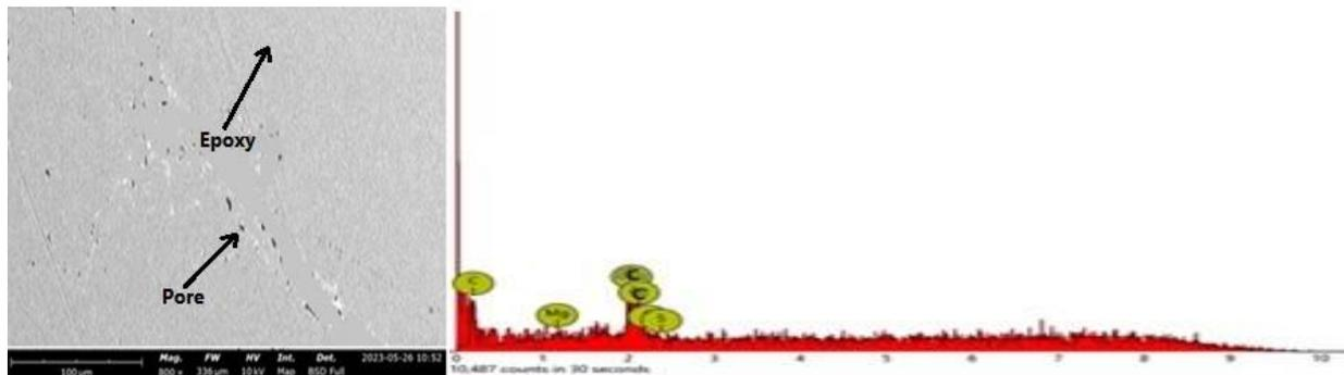
**Figure 3.** SEM and EDX spectrum of the control (unreinforced) sample A.
