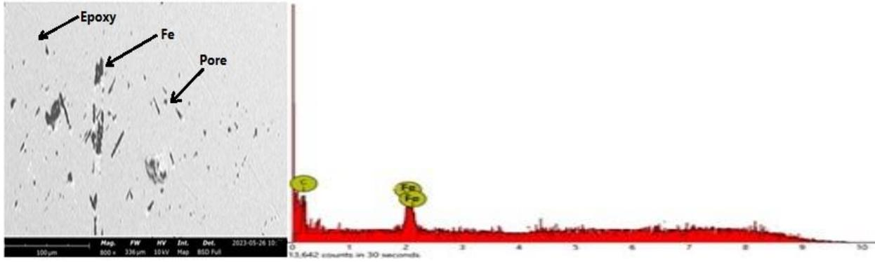
Figure 5. SEM and EDX spectrum of sample C.
