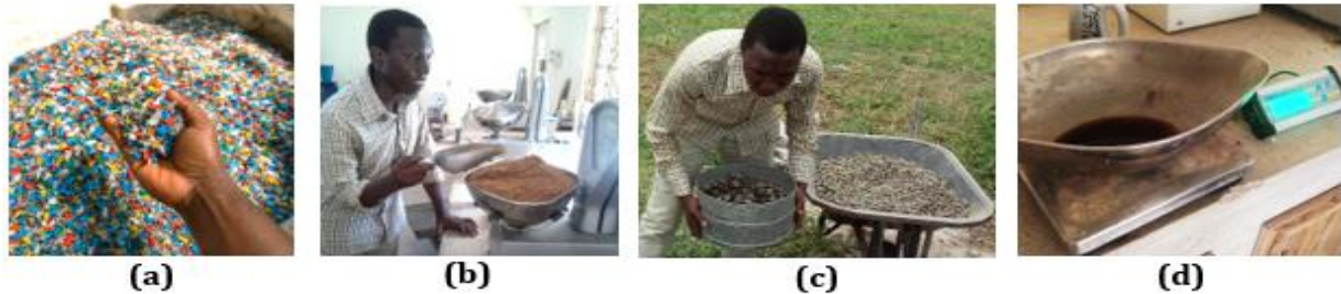
Figure 1. Concrete Materials (a) Recycled Plastic Aggregate (b) Fine Aggregate (c) Coarse Aggregate (d) Polycarboxylic Acid
