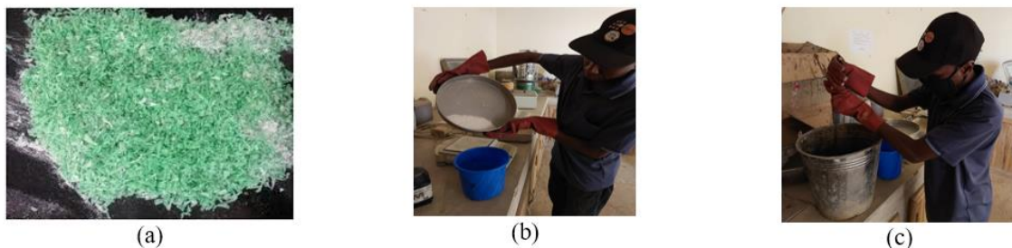
Figure 2. Process of Treating Recycled Plastic Aggregate (a) Recycled Plastic Aggregate Sample (b) Dissolving \text{Ca}(\text{ClO})_2 in Water (c) Soaking RPA in Solution
