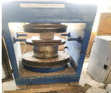
Figure 4. Compressive strength test.
