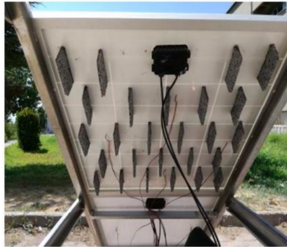
Figure 2. Mounted aluminium foam fins in the back panel (Selimefendigil et al., 2019)
