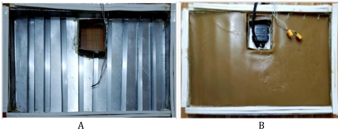
Figure 16. A) Container without PCM, B) Container with PCM. (Yousif and Kassim, 2023)
