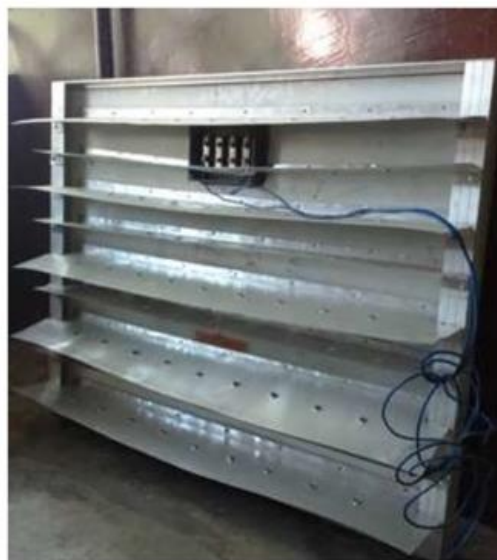
Figure 8. Backside of the PV panel with Fins. (Gotmare et al., 2015) .
