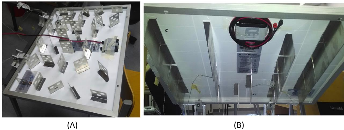
Figure 9. A) Randomly oriented and perforated Al-fins on backside surface of PV panel B) oriented parallel Al-fins on backside surface of PV pane. (Grubišić-Čabo et al., 2018)
