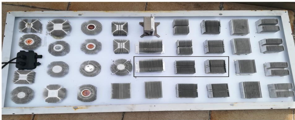
Figure 6. Back side of the passively cooled panel with heat sinks of different shapes and three investigated heat sinks marked with a black rectangle. (Krstic et al., 2024).
