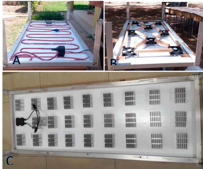
Figure 24. A) closed loop water cooled system, B) arrangement of fans for an active air-cooled system, C) solar panel with heat sinks. (Khan et al., 2017)
