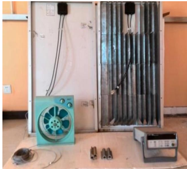
Figure 7. PV panels with and without cooling fins. (Chen et al., 2014) .
