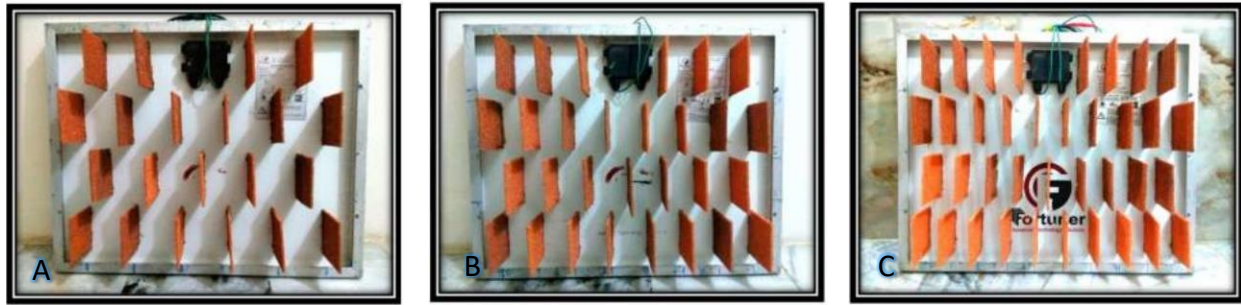
Figure 12. Staggered metal foam fin configurations. (A) First configurations. (B) Second configuration. (C) Third configuration (Hasan and Farhan, 2020) .
