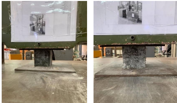
Figure 3. Compressive Strength Test
